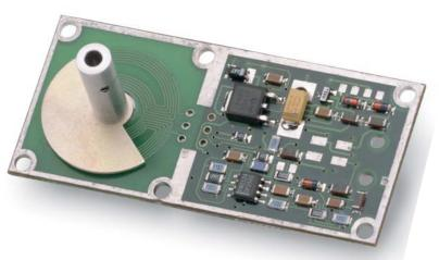
calibration and automated testing assures a nonlinearity error of less than  $\pm 0.5\%$  of full scale.
